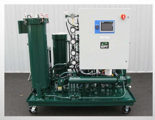
Two ICB IX cartridges, two ECR<sup>TM</sup> electrostatic collectors, a 6" x 18" 3 micron filter, TMR<sup>TM</sup> N2 (dry nitrogen) unit and heater.
